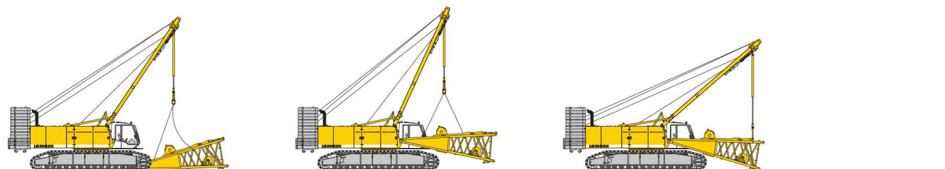
Unloading and assembly of boom foot
