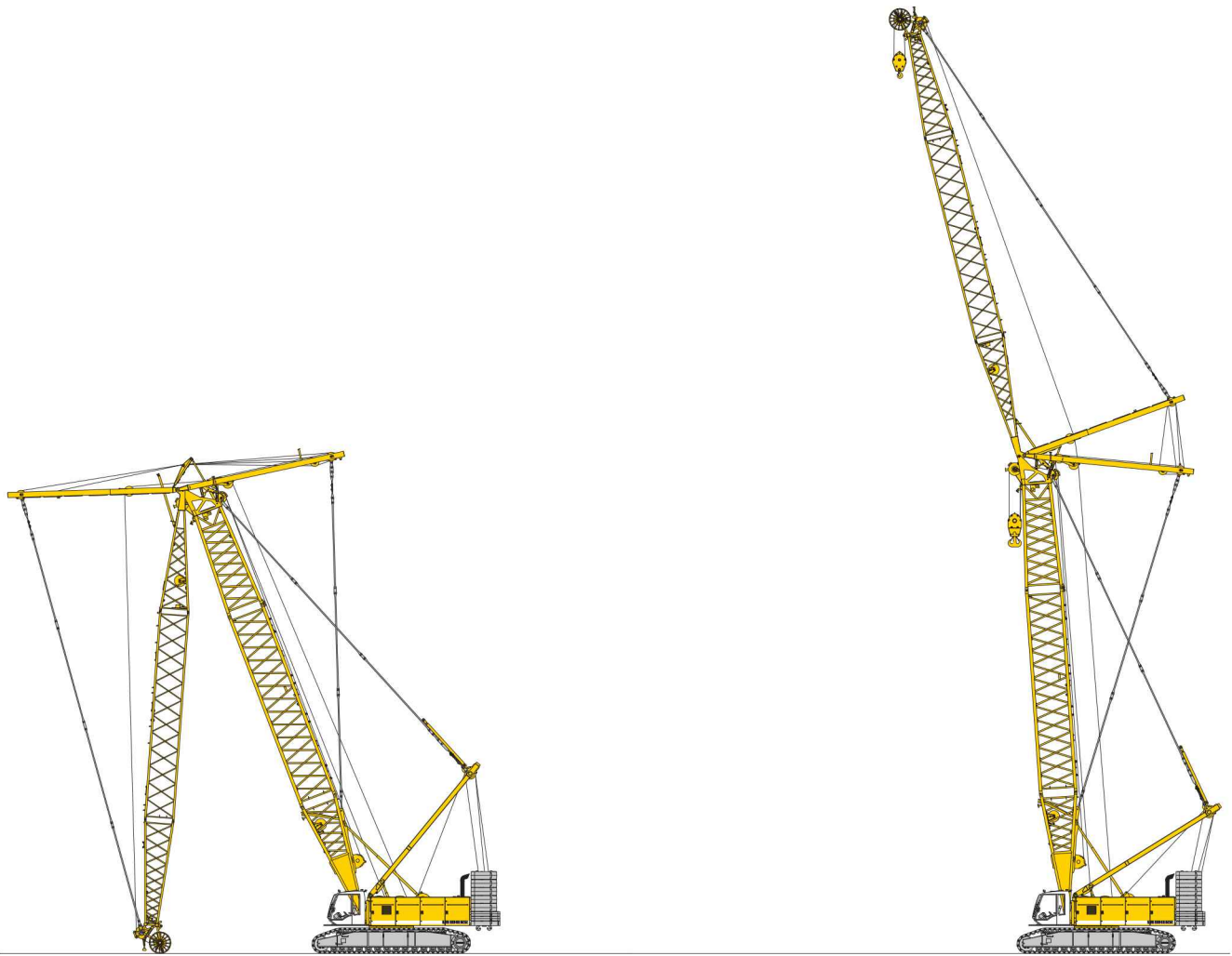
Erecting of main boom and luffing jib
