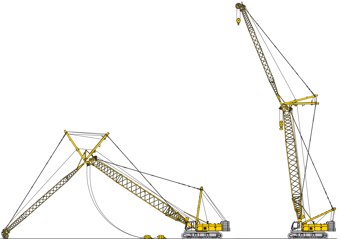
Erecting of main boom and luffing jib
