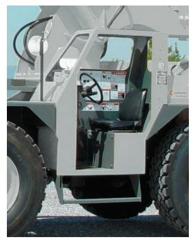
Standard: Open air cab shell w/overhead safety
